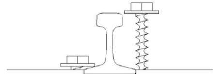
When installing track screws at a joint between two pieces of rail the tie should be centered below the joint. The track screws should all be placed on one side of the joint to allow the joint to be disassembled. Use care in locating these track screws so that they do not interfere with the installation of the bolts and nuts that hold the joint bars.
